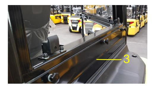
5. Seal marked edges using silicone
