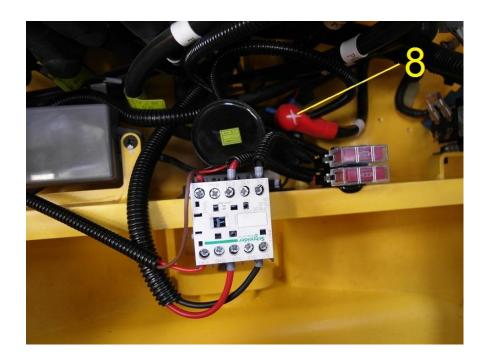
7. Connect the positive wire of heater electric bundle on the point (8)
