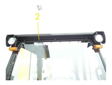
4. Screw the upper metal sheet (2) to the original holes using M8x20 screws
