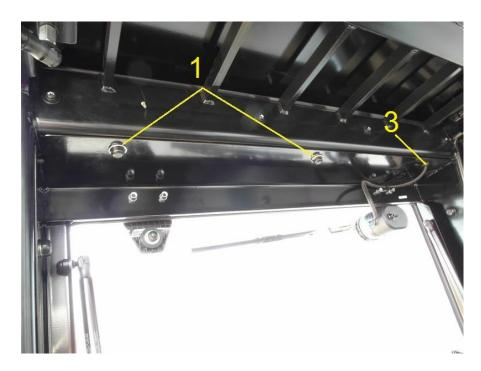
3. Put the rear panel between the rear profiles of the OHG and screw it with 2 screws HM10x25 and 2 screws M8x20
