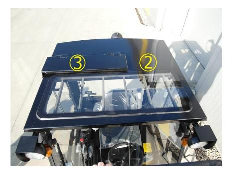
2. Put the roof (2) on the of OHG and place the following passage for access to batteries (3). Put the lateral gap equal.
