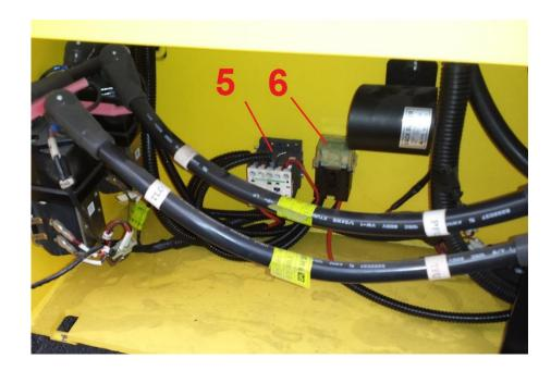
6. Set in the bottom of the compartment (4), the relay (5) and the fuses (6)
