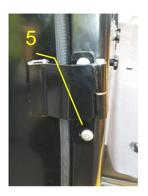
6. Put end set doors on the hinges. Adjust the doors position on such way that the gap between the seal and the inner OHG cavity was equal. Tighten the hinges screws
