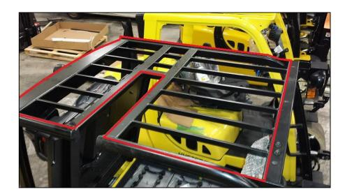
2. Put the roof (2) on the of OHG and place the following passage for access to batteries (3). Put the same lateral gap.
