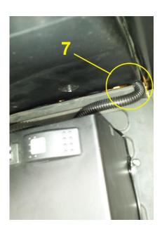
7. In the compartment (4), connect the positive beam heating on the point (8)
