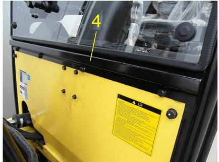
7. Screw the lower front sheet (4) to the OHG original holes using M8x20 screws
