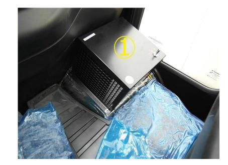
4. Screw the heater with M6 nuts
