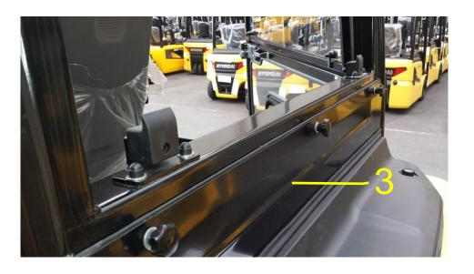
5. Seal marked edges using silicone
