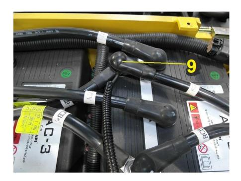
8. Connect the negative wireàf heater electric bundle (black wire) on point (9) (located at the rear of battery box)
