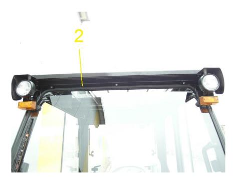
4. Screw the upport front sheet (2) to the original holes using M8x20 screws
