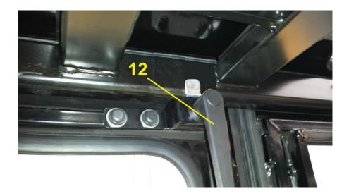
15. To block the top of the rear door part, just turn the lock (12)
