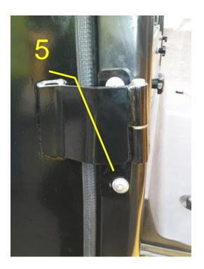
6. Put end set doors on the hinges. Adjust the doors position on such way that the gap between the seal and the inner OHG cavity was equal. Tighten the hinges screws
