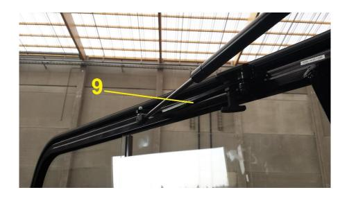
15. Screw the gas spring on the door support (9) with M8 nut
