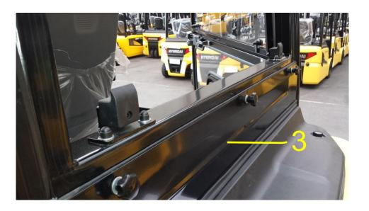
5. Seal marked edges using silicone
