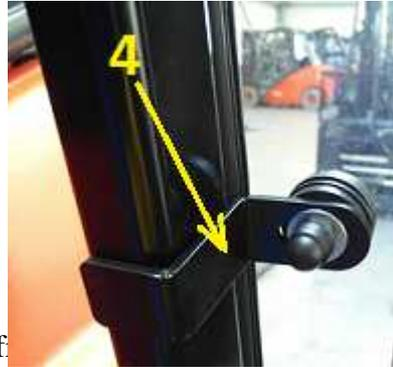
3. Prepare assembly set that is used for front glass/pane with assembly holders (4) to front profiles of OHG in such way so this glass is directly and evenly adhered to front upper and lower beam. Assembly holders to OHG using M8x25 screws.
