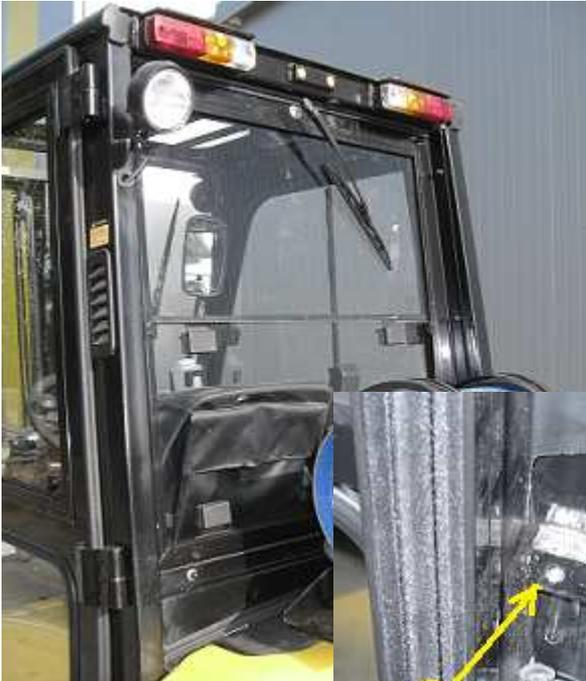
1. If holder of reduction of gas-fitting (1) is on inner part of rear profile of OHG move this holder of reduction of gas-fitting one step backwards so hoses of gas-fitting do not clash with rear panel. Put rear panel to OHG in such a way that top panel seal adheres inner edge of rear upper profile of OHG evenly. Cut part that is in lower part of OHG should adheres inner side of holder of reduction (2) evenly
