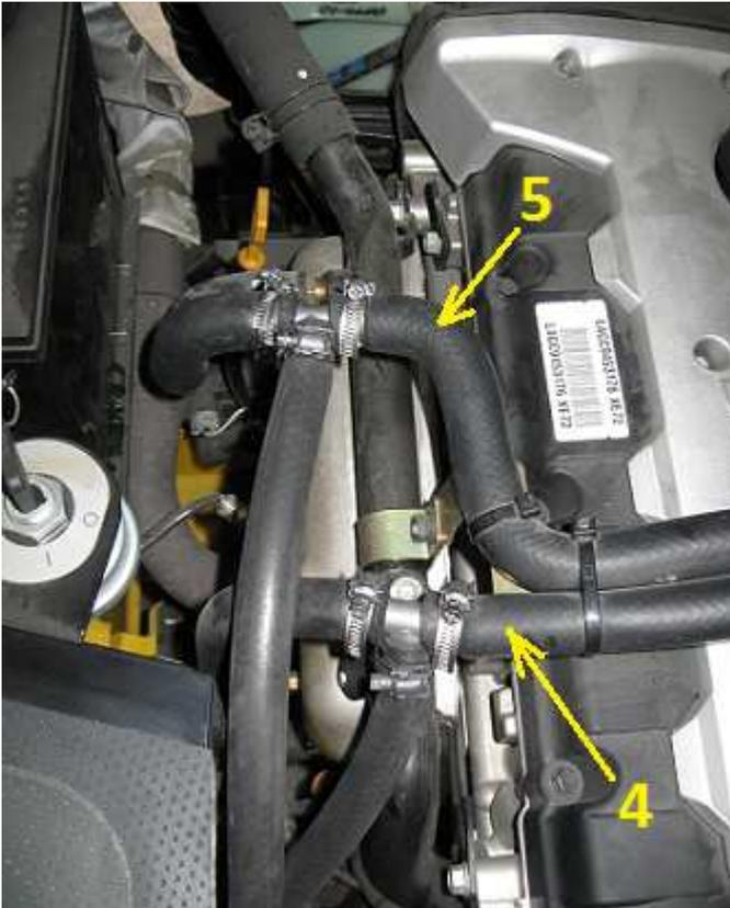
2. Assembly T-pipe with hose that supplies heating staff to heater together with cut hose (4).
