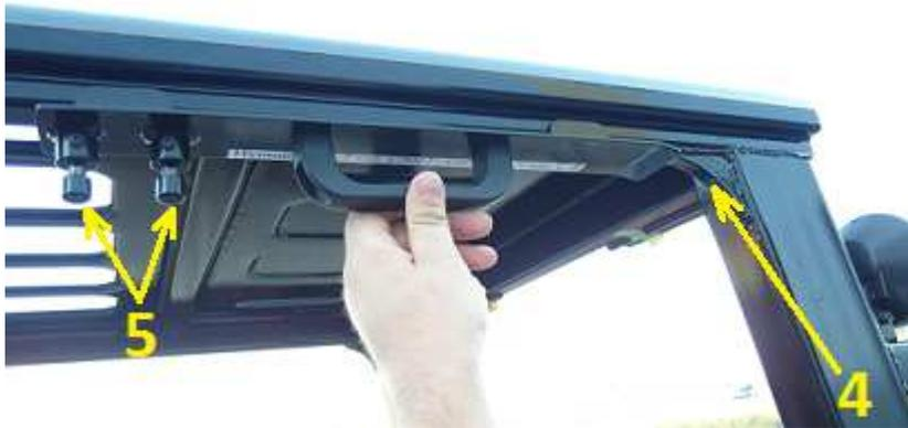
Remark: this tool must be pushed to interior of cab firmly. Mark assembly holes for holders of gas spring by hitting in bolts (5). Drill holes  $\varnothing 11$  in these places and then set blind rivet nuts M8. Assembly holder of gas spring (6) using M8x20 screws.
