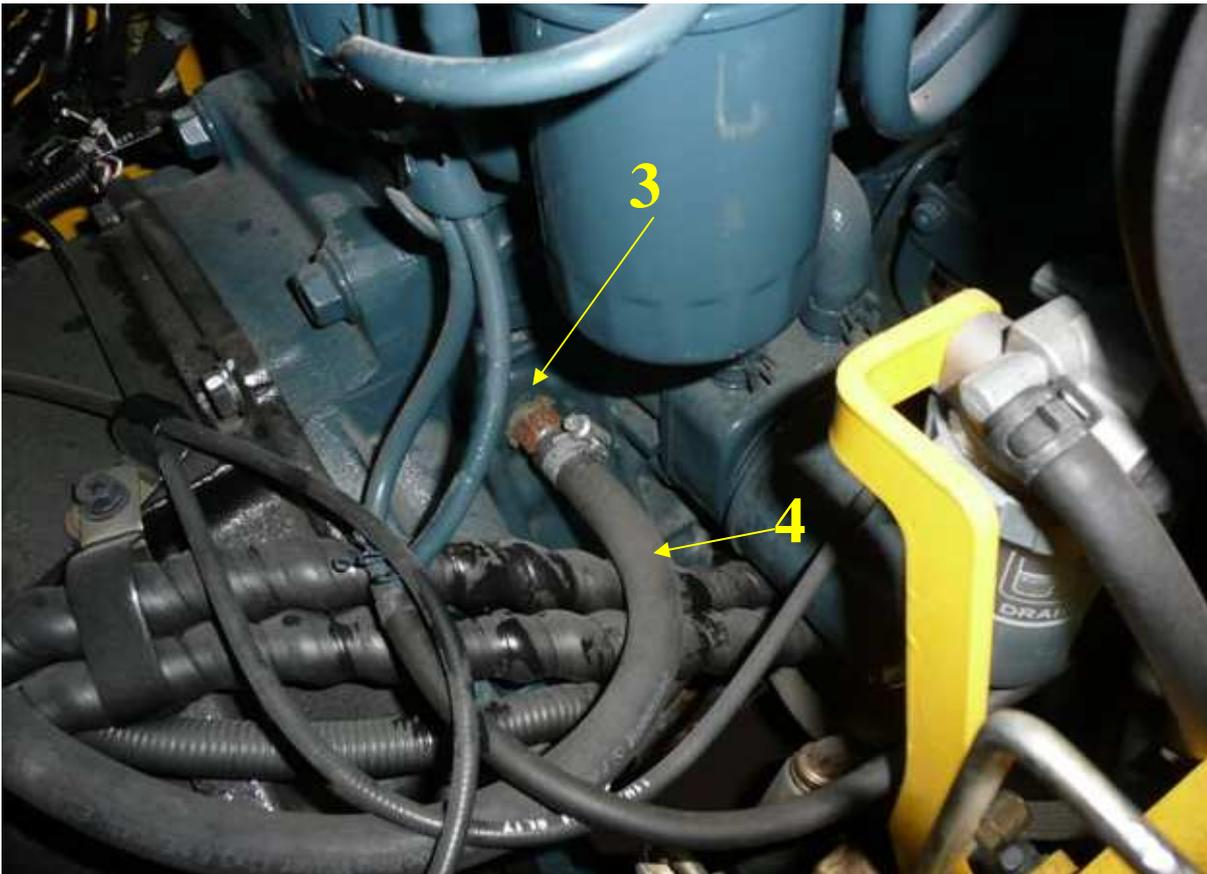
4. Match reduction and then screw it together with copper cushion (washer) in. Then assembly reduction (4) together with hose, that supplies heating staff to heater.
