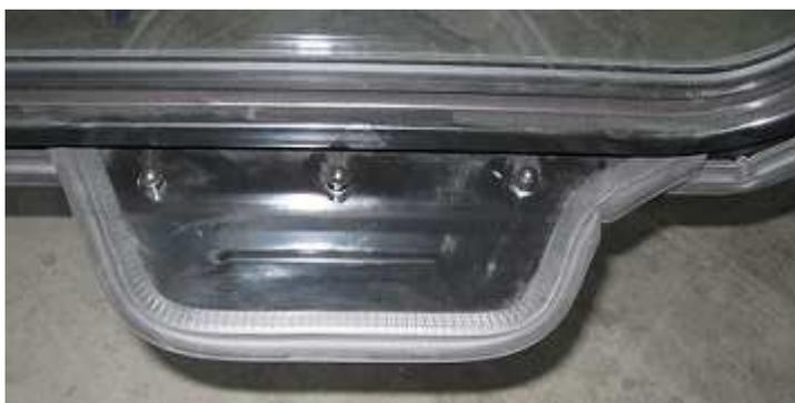
4. If there is any gap between floor of door and floor of forklift when door is closed, floor of door must be regulated by pushing it on bean-shaped holes to get rid of this gap.
