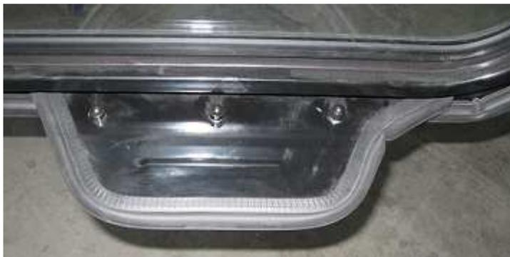
10. If there is any gap between floor of door and floor of forklift when door is closed, floor of door must be regulated by pushing it on bean-shaped holes to get rid of this gap.
