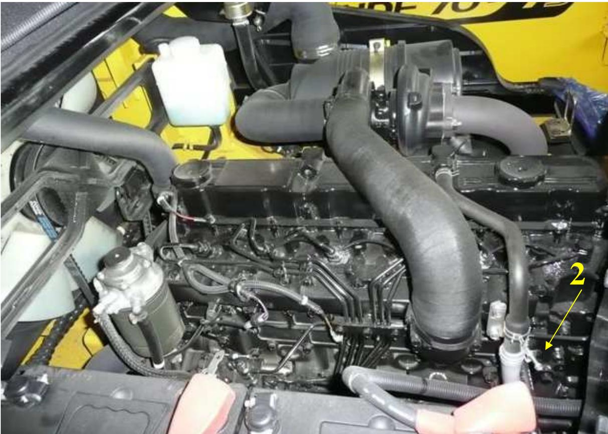
4. Match reduction and then screw it together with coppery cushion (washer) in. Then assembly reduction together with hose, that supplies heating staff to heat
