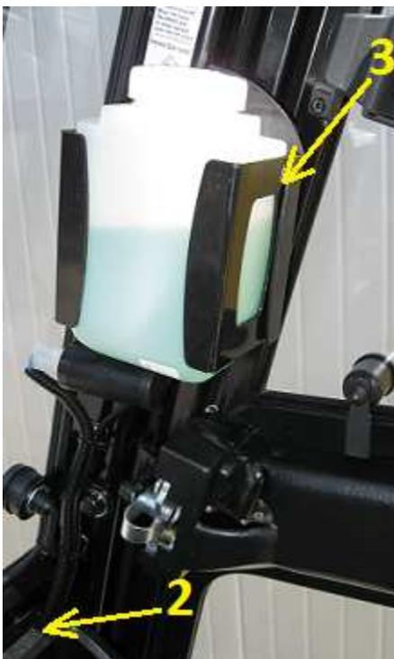
5. Drill  $\text{\O} 20$  hole in right top part of cockpit (2). Draw sprinkler hose under cockpit towards right front profile.
