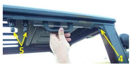
Remark: this tool must be pushed to interior of cab firmly. Mark assembly holes for holders of gas spring by hitting in bolts (5). Drill holes Ø11 in these places and then set blind rivet nuts M8. Assembly holder of gas spring (6) using M8x20 screws.
