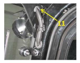
15. Draw decoupled wires of front lamps through holes in front upper bar (11) and plug them back in.
