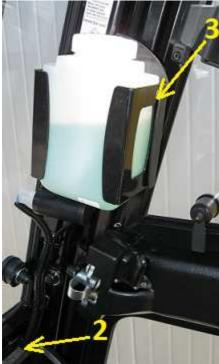
5. Drill Ø 20 hole in right top part of cockpit (2). Draw sprinkler hose under cockpit towards right front profile.
