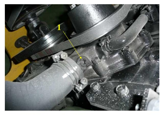
2. Match reduction and then screw it together with coppery cushion (washer) in. Then assembly reduction together with hose, that takes heating staff out of heater.
