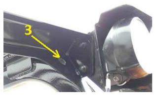
2. Decouple wires of front lamps before assembly of front upper beam. Screw front lamps with their covers out. Put front upper metal beam (2) against OHG in such a way that top part of the bar adheres to front inner part of forklift roof frame. Assembly front upper beam to side part of OHG using original screws together with covers of lamps. Draw wires of front lamps trough hole (3) that is in front upper beam.
