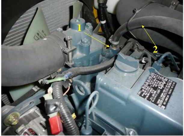
2. Match reduction and then screw it together with coppery cushion (washer) in. Then assembly reduction (2) together with hose, that takes heating staff out of heater.
