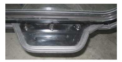
10. If there is any gap between floor of door and floor of forklift when door is closed, floor of door must be regulated by pushing it on beanshaped holes to get rid of this gap.
