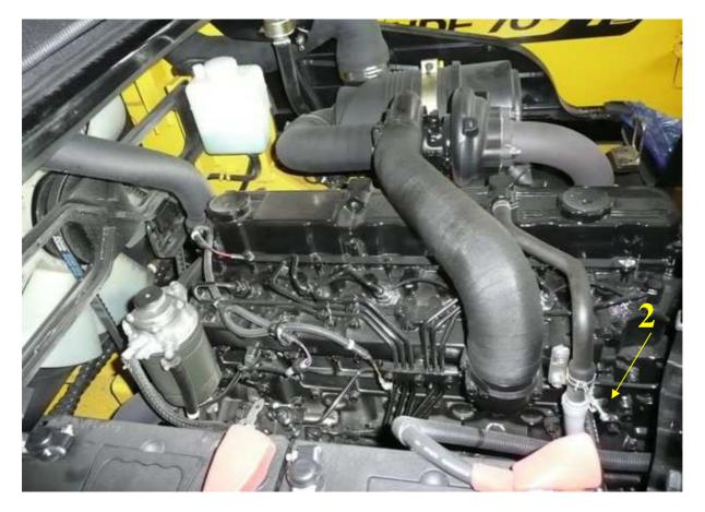
4. Match reduction and then screw it together with coppery cushion (washer) in. Then assembly reduction together with hose, that supplies heating staff to heat
