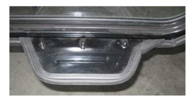
4. If there is any gap between floor of door and floor of forklift when door is closed, floor of door must be regulated by pushing it on bean-shaped holes to get rid of this gap.
