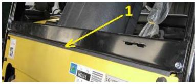
1. Put front lower beam to OHG in such way so lower part this beam is directly and evenly adhered to front part of cockpit (1).
