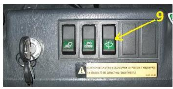
14. Assembly front wiper switch on cockpit to the right side of steering column (10).
