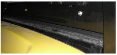
2. Assembly rear lower beam to outer lower part of rear frame using M6x20 screws.
