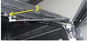
8. Mark assembly holes looking at (taking care of) holder of gas spring on OHG. Drill holes Ø11 and set blind rivet nuts M8 in these places.
