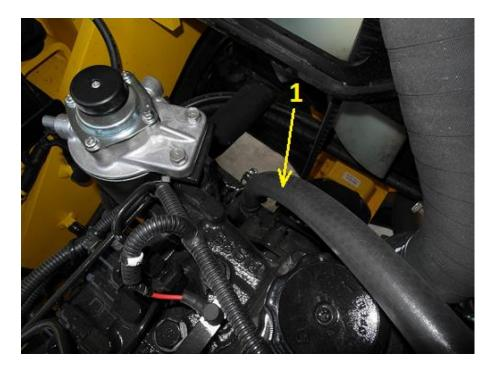
3. Screw protective screw from side part of engine body out.
