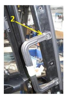
5. Screw holder (2) out and assembly it ca. 100 mm below its original position so holder of front sliding glass of door does not hit this holder when door is shutting.
