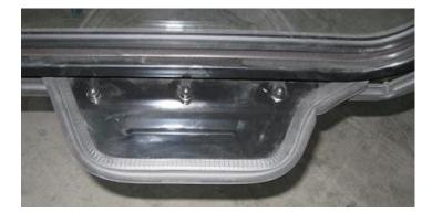
11. If there is any gap between floor of door and floor of forklift when door is closed, floor of door must be regulated by pushing it on beanshaped holes to get rid of this gap.
