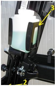
5. Drill  $\emptyset$  20 hole in right top part of cockpit (2). Draw sprinkler hose underneath cockpit towards right front profile.
