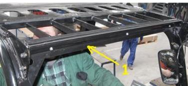
Drill holes Ø7 in marked places. Assembly upper front beam to OHG using M6x25 screws
