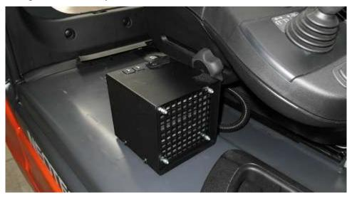
2. Embed M6 blind rivet nut into the original hole (placed in the forklift counterweight). Screw the contactor (1).
