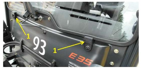
3. Lean the front glass on the holders (1) and then screw the upper part of the front glass/pane to the original holes using M8x45 screws.
