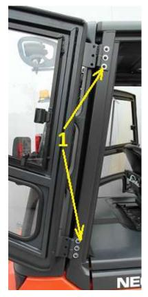
2. Embed M8 blind rivet nuts into original holes. Screw the lock pin holder (2) using M8x25 screws.
