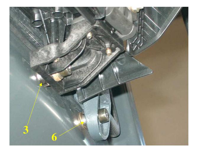
2. Put M8 blind rivet nuts in the openings in the truck frame, slightly fasten the holders (4) which fix the rear window, using M8x35 bolts (5) together with  $18/\emptyset$  9 spacing sleeves (6).
