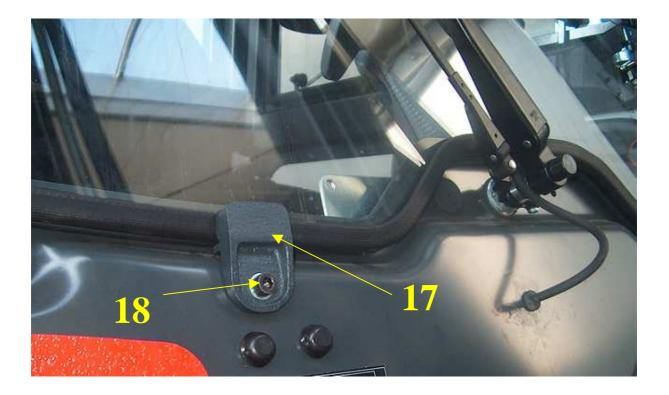
3. Rest the windscreen on the fixing holders and fasten it using M8x45 bolts (19).
