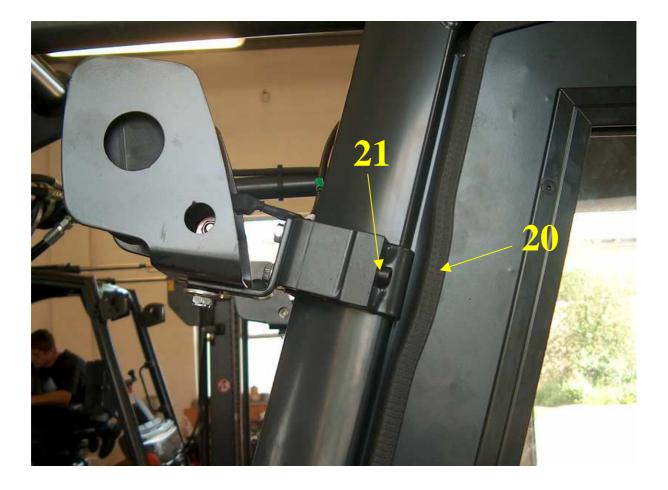
2. Put the halogen lamp fixture against the original opening in the truck frame and mark the point for the M8x15 bolt. Drill Ø9 opening at the marked point.3. Attach the halogen lamp fixture with M8x15 bolts (22).
