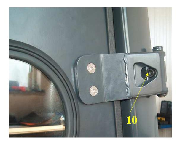
3. Ream the Ø9 openings ( 11 ) to obtain Ø11 diameters, and place the M8 blind rivet nuts inside.
