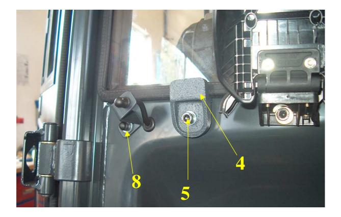
3. Rest the rear window on the fixing holders and fasten the window using M8x45 bolts (7).
