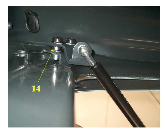
5. Mount the gas spring to the ball pins.
