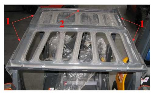
2. Put roof to upper part of OHG so this roof is on this frame evenly. Assembly rear part and middle part of this roof using self-drilling Ø6,3x32 screws. Assembly front part of roof (4) with front upper beam (of front panel) using self-drilling Ø4,8x19 screws.
