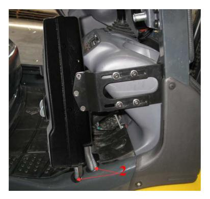
3. Assembly this heater to its holder back. Draw hoses in direction of chamber of engine.
