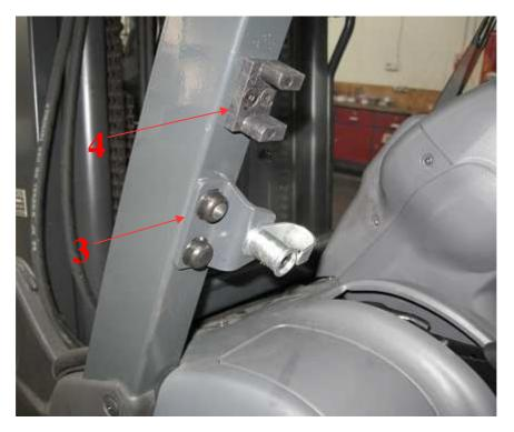
8. If there is any gap between floor of door and floor of forklift when door is closed, floor of door must be regulated by pushing it on bean-shaped holes to get rid of this gap.
