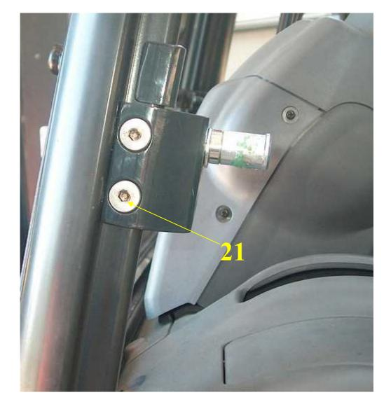
7. Put the side profile to the forklift frame, mark places for assembly holes.
