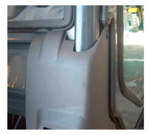
3. Fasten the front lower beam (4) using M10 screws (3) to the frame of the forklift.
