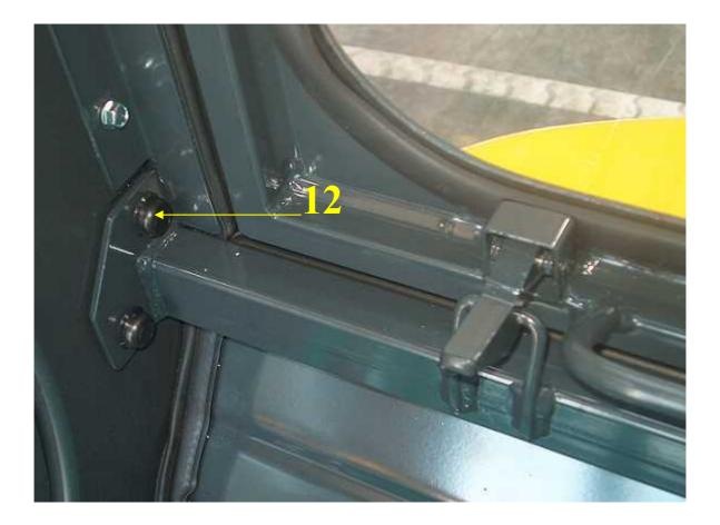
5. Put rear-side angles profiles to the forklift frame and then fasten them to this frame using self-drilling screws  $\emptyset$  6,3x25 (13). Assembly gas springs to ball pins.
