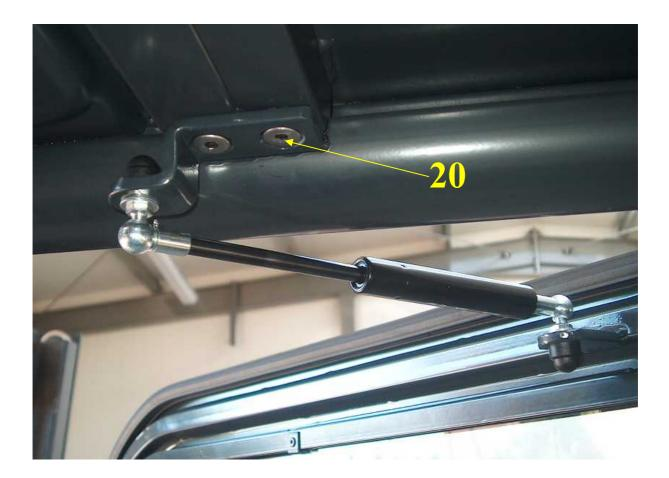
6. Press the door to the forklift frame, try the holder of the lock latch and mark places for assembly holes on the forklift frame. Drill holes  $\emptyset$ 11,2 in marked places and set blind rivet nuts M8. Fasten the holder of the lock latch suing M8x25 screws (21)
