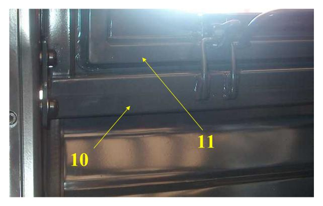
4. Drill holes  $\emptyset$  11 in marked places, set blind rivet nuts M8 and fasten the lower beam to the forklift frame using M8x25 screws (12).
