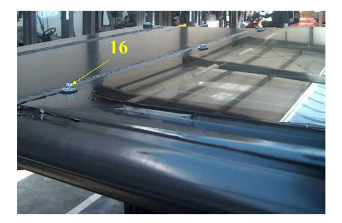
3. Put the rear metal plate of the roof to the forklift frame, mark the place for holes from these holes that are on the foklift frame. (17). Drill holes in marked places, then put the silicone onto the forklift frame and fasten the plate using M8x20 screws (18)
