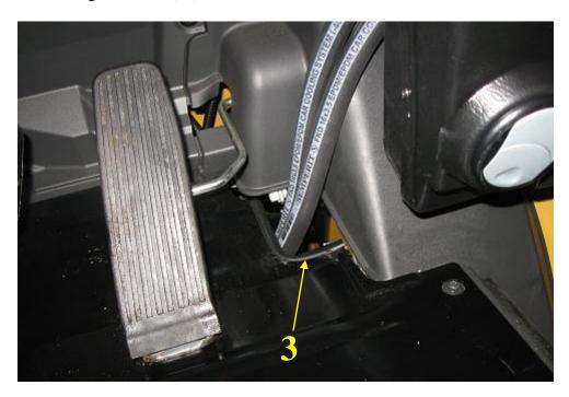
7. Cut hoses (4) and (5) into 2 pieces. Attach heater inlet hose to cut hose no (4) and heater outlet hose to cut hose no (5).
