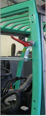
V. Coapt the floor of the door so it should fit to the forklift frame steadily usin 3 screws like is marked on the photo
