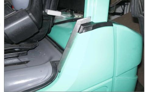
II. Set blind river nuts M8 in the holes in the frame of the forklift.
