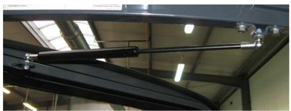
IX. Fasten the holder to the forklift frame using M8x20 screws.
