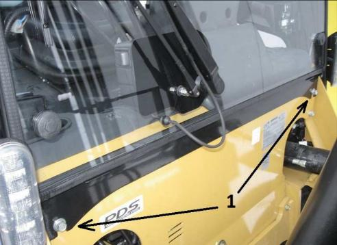
III. Complete assembly kit of front glass according to drawing : 1. Screw M8x25.
