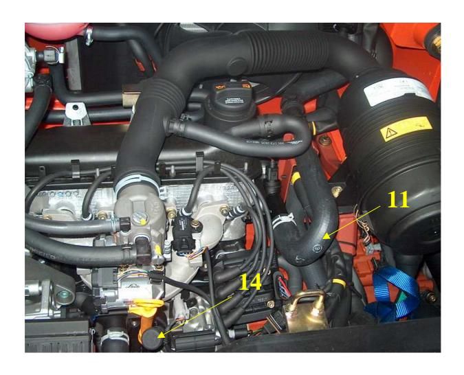
9. Install the copper T-pipe (12) in the cut hose using bands. Connect hose (13) to the T-pipe, which supplies the heating medium to the heater. Connect hose (15) to the connector pipe (14) which discharges the heating medium from the heater.
