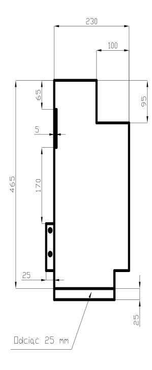
4. Weld the sheets (3) and (4) as shown in the drawing.
