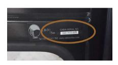
On the identification plate, mounted on the inside of the right door (for a complete rigid cabin) or on the inside of the roof (for all other cabin module types)
