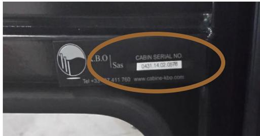
*On the identification plate, mounted on the inside of the right door (for a complete rigid cabin) or on the inside of the roof (for all other cabin module types)*
